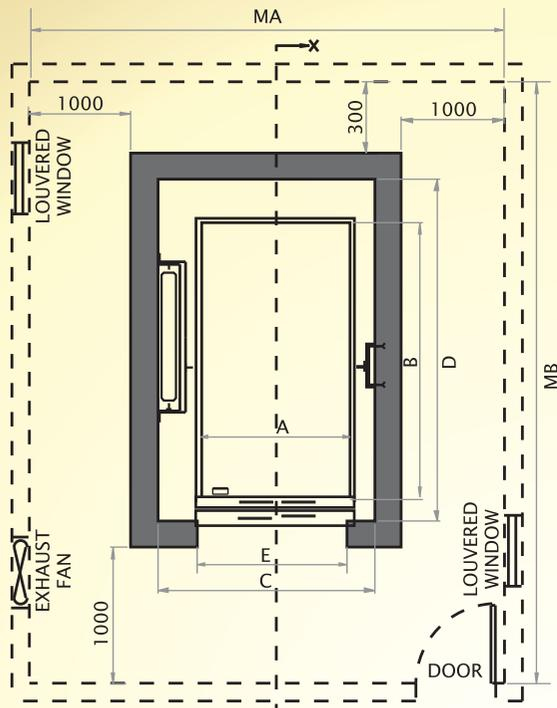
LIFT SHAFT, CAR, C.W. & MACHINE ROOM PLAN
